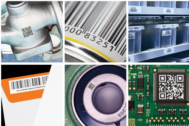
Figure 1. Industrial barcodes appear on a variety of surface types and in varying sizes. To better accommodate this broad range of barcodes, scanners need new types of CMOS image sensors.
